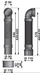
**WC connection pipe DN 90/DN 100, flexible,
