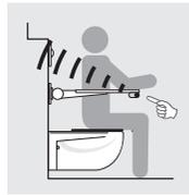
**WC control system using encoded radio signals for accessible construction as per DIN 18040**
