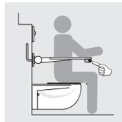
**WC control system, 2-cable, for accessible construction as per DIN 18040**
